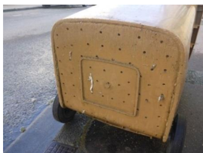
Photo 6 Custom-made filtration systems in a bin with a perforated base (source Cedre)
