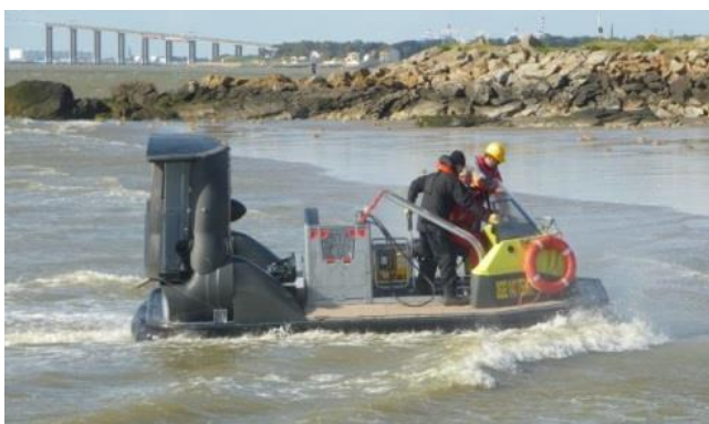
Photo 28 Prototype of hovercraft for operations on mudflats and in shallow waters ("Hoverspill" CE project, 2009-2013) (source Cedre)
